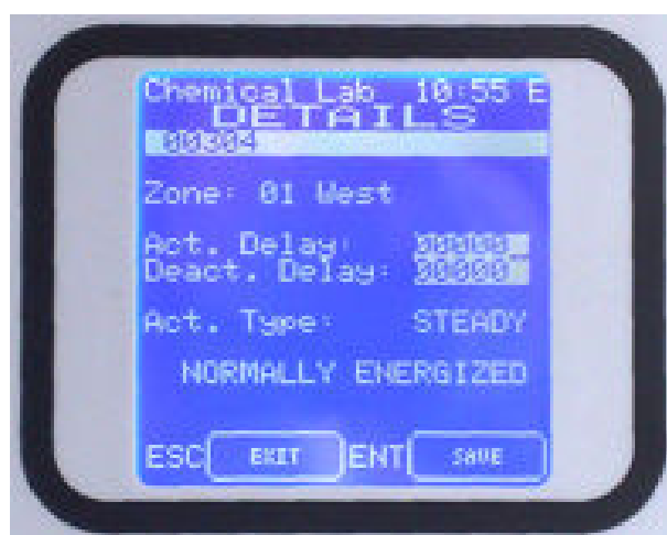
Fig. 3.8.3 b) Output details screen in “Engineer” level
