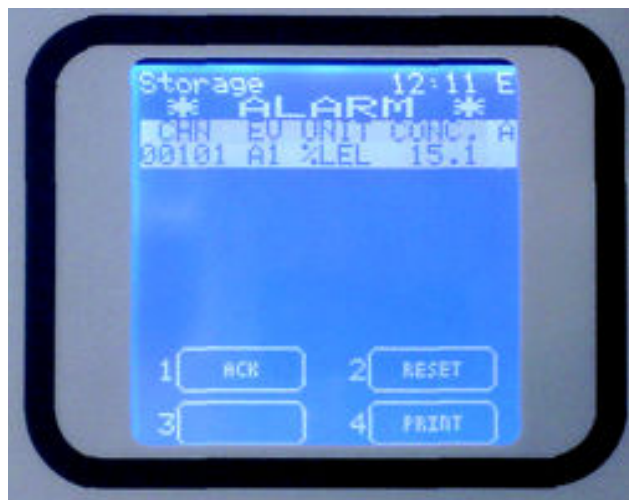
Fig. 3.5.1 b) Active Events screen with alarm only
